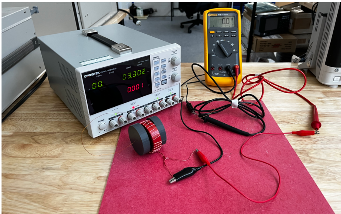
Polarity Testing – DC Voltage. Typical Test Setup: Magnesil Current Transformer.
